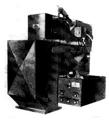
Thayer filling scale for net weighing of granular, flake pellet, or fibrous materials. The unit handles up to 5 bags per minute of any desired weight from 25 to 200 lb. The machine is designed for use in automatic weighing and filling lines
